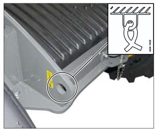
(fig.156/C) Front anchorage point
