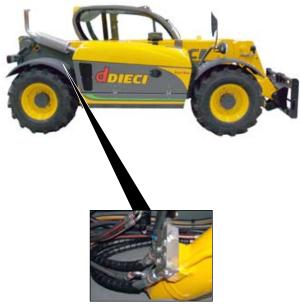
(fig.74/D) (Boom raising cylinder block valve)
