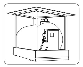
5. The delivery tap must be larger at the bottom to trap any deposits; it should also be equipped with a removable filter. The tank must be tilted by 40 mm per metre towards the sediment drain plug. 6. Fuel barrels (see the figure below) must be stored under cover to prevent water seepage. The barrels should also be tilted slightly, to allow any water to drain off the upper rim. The fuel barrels must not be stored for too long before being used.
