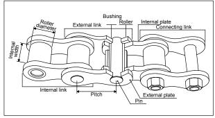
(fig.91/D) Components of a standard chain
