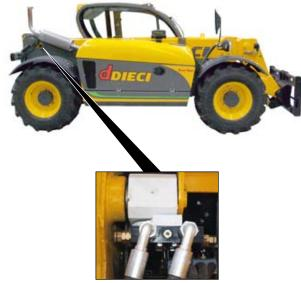
(fig.75/D) (Boom internal extension cylinder block valve)
