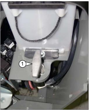
(fig.1/D) Routine work position - Closed circuit
