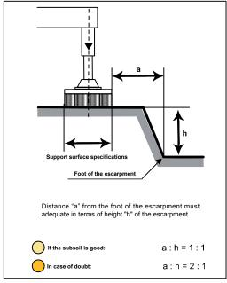
(fig. 5/B) Machine positioned on an escarpment
