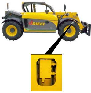
(fig.76/D) (Swivel plate cylinder block valve)
