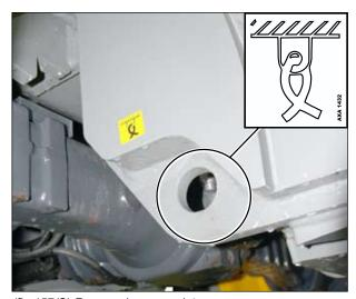
(fig.157/C) Rear anchorage point
